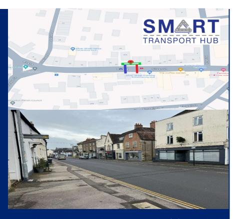
STH carried out a 7-day ATC on B3414 Silver Street commencing the 07/12/23. The number of vehicles exceeding the speed limit of 30mph was 2968 which is 4.24% of the total vehicles recorded in both directions which was 69970.
