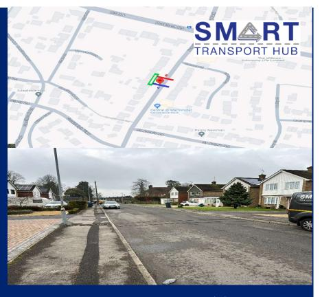
STH carried out a 7-day ATC on Prestbury Drive commencing the 07/12/23. The number of vehicles exceeding the speed limit of 30mph was 442 which is 3.46% of the total vehicles recorded in both directions which was 12771.
