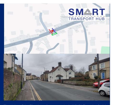
STH carried out a 7-day ATC on Vicarage Street commencing the 29/01/24. The number of vehicles exceeding the speed limit of 30mph was 2783 which is 6.47% of the total vehicles recorded in both directions which was 43023.
