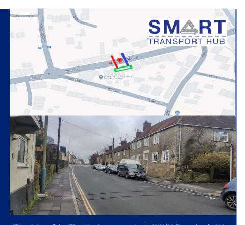
STH carried out a 7-day ATC on West Street commencing the 29/01/24. The number of vehicles exceeding the speed limit of 30mph was 2115 which is 6.41% of the total vehicles recorded in both directions which was 32979.
