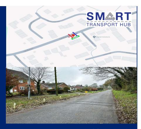
STH carried out a 7-day ATC on Bradley Road commencing the 07/12/23. The number of vehicles exceeding the speed limit of 30mph was 658 which is 24.08% of the total vehicles recorded in both directions which was 2733.
